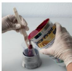
3. Pour the necessary quantity of ink into the Teca-Print mixing cup.
