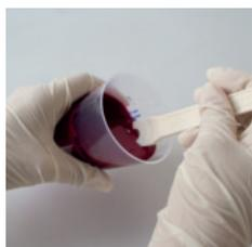
5. Hold the cup so that the large round opening of the Viscospatula is halfway submerged in ink.
