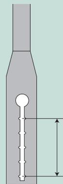
With a watch or while counting the seconds (3-4-5...) the time the ink needs to flow off the measuring distance can be determined.
